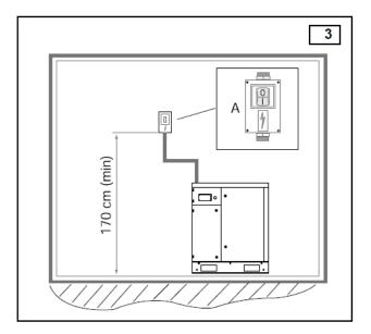
**N.B.** To determine the cables cross-section and the type of switch, refer to the data reported on the technical table. Sizing according to "VDE 0100, Part 430 and 523", star-delta starter, 30° C ambient temperature and cable length lower than 50 meters.
